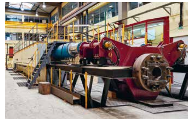
Cable fatigue bench.
